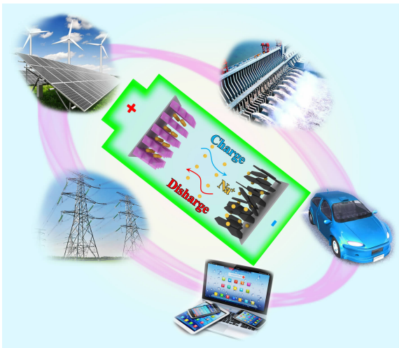
图 1 钠离子电池的工作原理及潜在用途 Fig. 1 Working mechanism and potential applications of sodium-ion batteries
