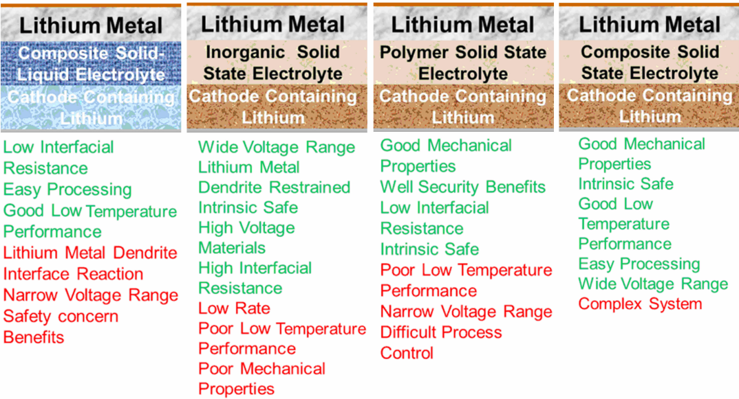
图 9 全固态锂电池的分类及特点 Fig. 9 The classification and property of solid state batteries
